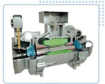
High power density, small size, light weight and compact structure; The motor adopts the refrigerant cooling technology. The low-temperature liquid refrigerant is sprayed from the compressor shell and evenly sprayed into the motor chamber through the flow-channel hole of the shell. The refrigerant evaporates and absorbs heat to take away the heat.
